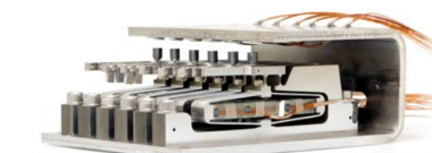
Fig. 5.m: Piezo activated arms (3 mm stroke) for X-ray filter holder 10 ms switching time
