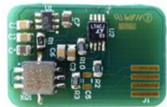
Fig. 9.l: Three axes accelerometer PCB mounted
