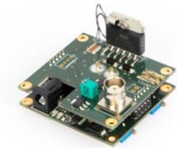
Fig. 8.s: OEM amplifier board for driving magnetic actuators
