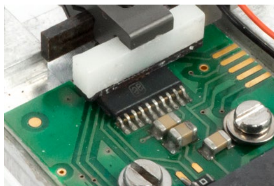
Fig. 9.k: Linear magnetic encoder (hall effect sensor)
