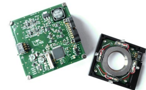
Fig. 5.k: Microscanning piezo XY stage (+/- 10 µm stroke) and its driver box for image resolution enhancement
