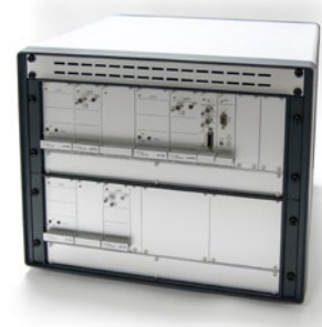
Fig. 8.o: Rack cabinet mounted LA75C push pull amplifier channels for driving large capacitance piezo mechanism
