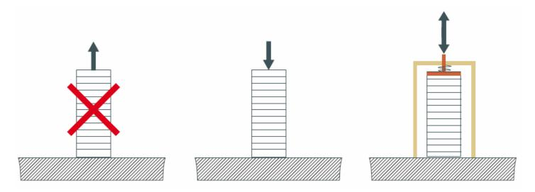
For linear actuators it is recommended not to use a metal plate on top and bottom in order to avoid short circuit.
