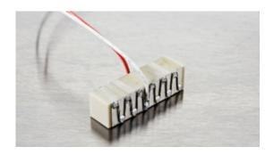
Noliac plate stack actuator NAC2015-Hxx (height in mm – Hxx) is based on the multilayer actuator NAC2015 and can be stacked to match you requirements. The standard range of NAC2015-Hxx is produced in a height between 4-100 mm. The plate stack provides a stroke up to 161.7  $\mu m$  and blocking force up to 4200 N depending on the height of the stack.
