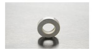
The Noliac piezo actuators can reach full performance at very low operating voltage. The ring actuator NAC2121 is the smallest of our standard ring actuators ranging only 6x2 mm with a free stroke of 3.3  $\mu$ m and a blocking force of 1060 N.
