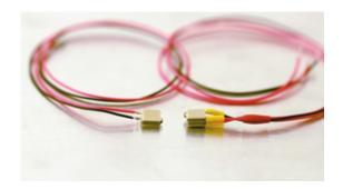
The Noliac shear stack NAC2402-H2.3 features shear motion on the X-axis. NAC2402-H2.3 measures 5x5 mm with a height of 2.3 mm and provides a free stroke of 3?m and a capacitance of 1.7 nF.
