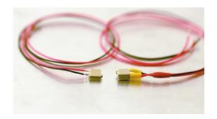
The Noliac shear stack NAC2403-H1.7 features shear motion on the X-axis. NAC2403-H1.7 measures 10x10 mm with a height of 1.7 mm and provides free stroke of 1.5 ?m and a capacitance of 3.3 nF.
