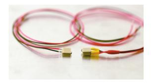
The Noliac shear stack NAC2903-H2.8 features shear motion on the X/Y-axis. NAC2903-H2.8 measures 10x10 mm with a height of 2.8 mm and provides a free stroke of 1.5/1.5 ?m and a capacitance of 3.3/3.3 nF.
