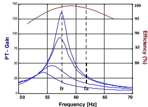
Frequency and load response of a typical piezoelectric transformer
