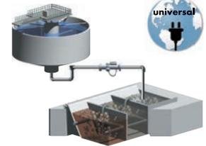
■ Measurement of concentration of sludge returned to aeration tank
