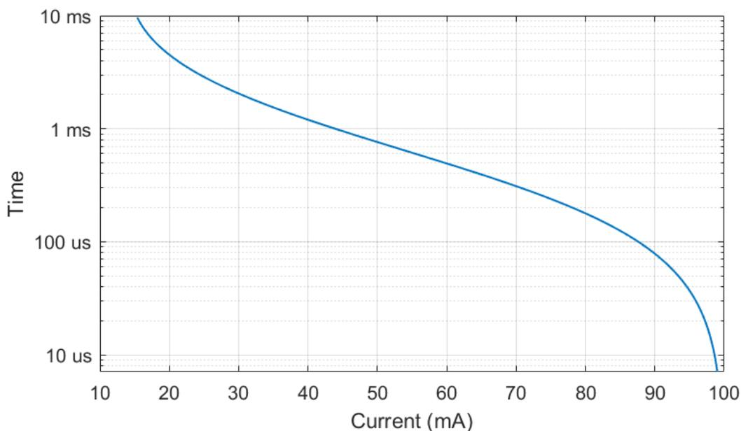
Figure 6. Peak current duration for the TD250.
