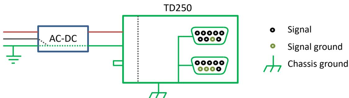
Figure 3. TD250 Chassis and signal ground configuration
