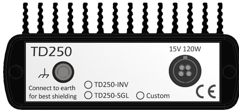
The rear panel includes a chassis earth connector that can be used to improve shielding, particularly when using an alternative power supply with an isolated output. This connector will accept a wire lug, 4mm plug, or stripped wire. The negative terminal of the power input connector is also connected to the chassis. Since the negative output terminal of the included power supply is connected to earth, the chassis is normally earthed.
